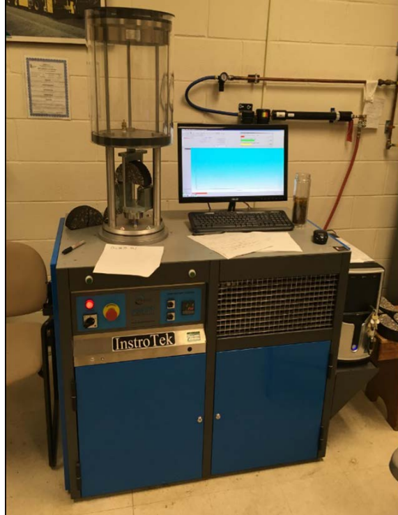
Figure 3.1: AMPT Machine for the IL-SCB Test
